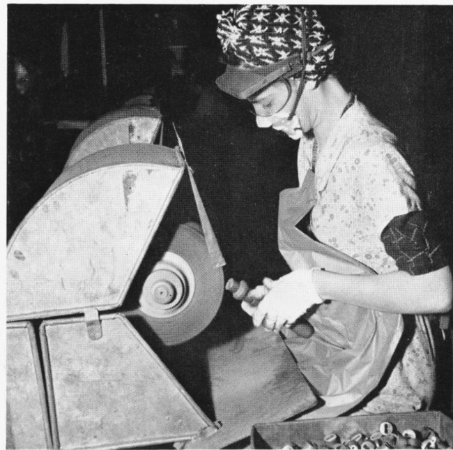
In this buffing operation, Mary Greguoli of the Buff Room is wearing safety cap and eye shield, dust mask and cotton gloves. Although a blower removes the dust, some particles fly from the wheel.
