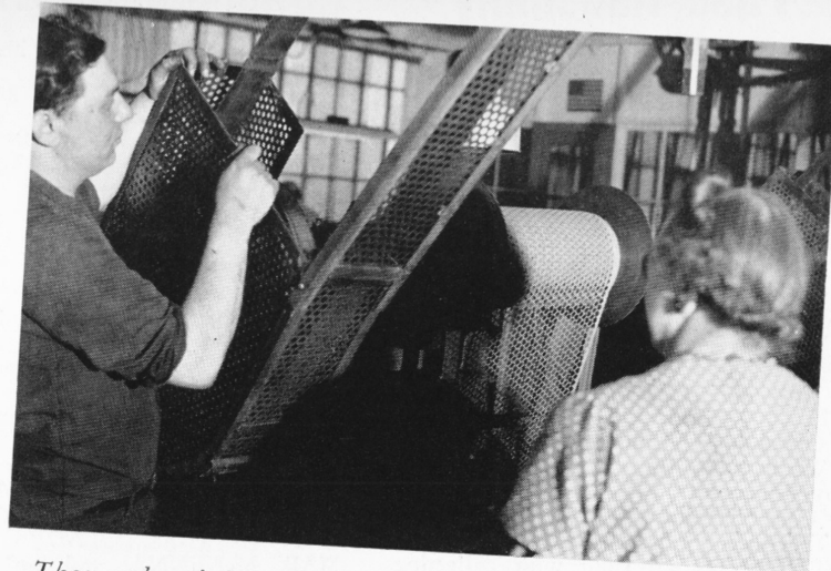
Thousands of large and small moving parts are guarded by metal shields. Anthony Masi of the Tin Shop is installing a guard in the Closing Room. Josephine Higgins, an operator in the Room, looks on.
